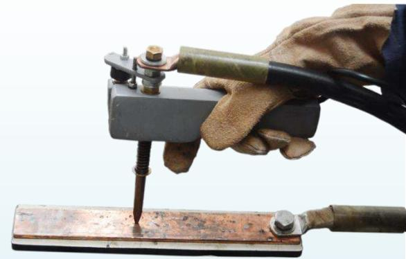
SINGLE SIDE SPOT WELDING FOR JOBS THAT ARE DIFFICULT TO WELD.
