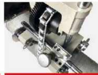
According to the size of the pipe diameter, increase or decrease the chain
