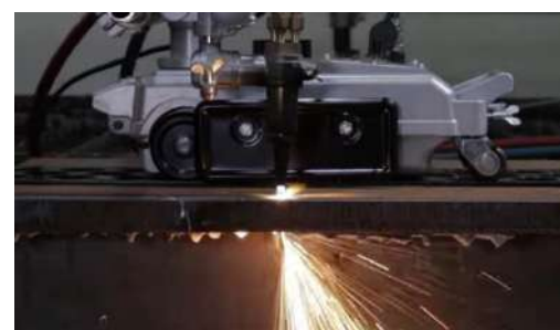
Right angle cut in 30mm metal
