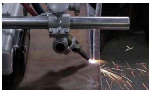
45 degrees cut in 30mm metal
