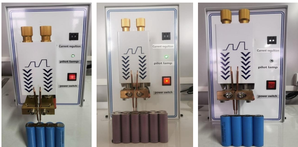
Welding head panel: pressure adjustment knobs (top), current regulation switches, pilot lamp, power switch and the two electrode holders
