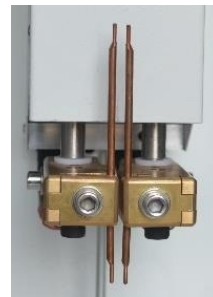
Electrode holders with Ø3 mm welding tips
