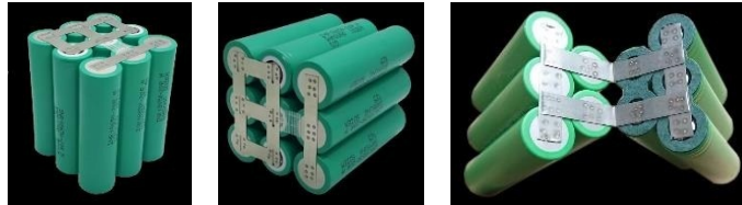
Welded samples - dual-pulse energy welding in milliseconds
