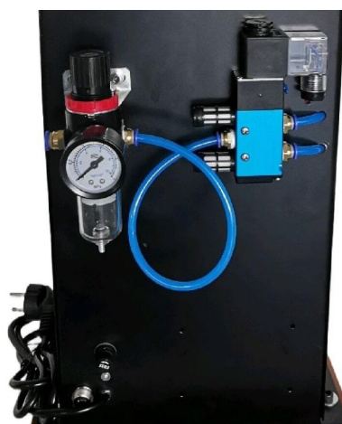
Side: air filter-regulator with gauge, solenoid valve and cylinder speed valves
