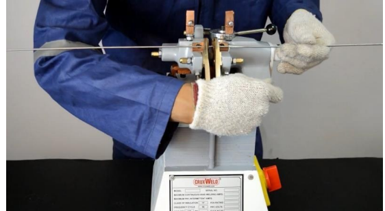
Welding a wire joint
