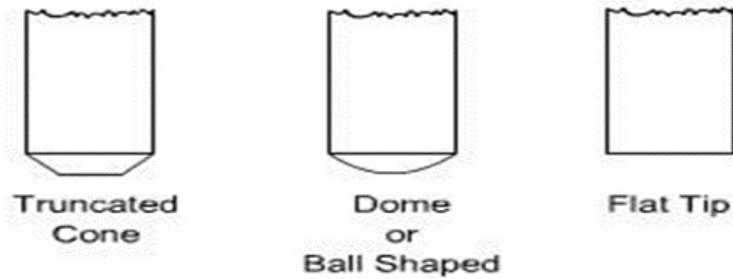
Fig. 4.3 Electrode tip shapes for spot welding
