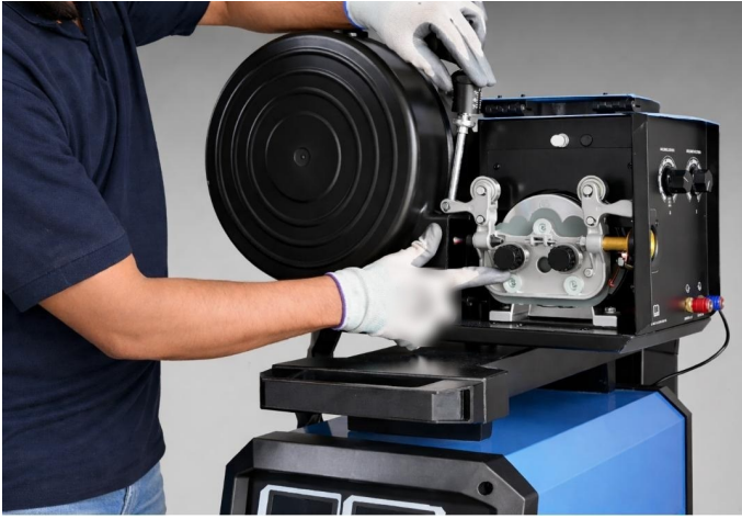
Fig. 5.4 4-roll wire drive with pressure arms
