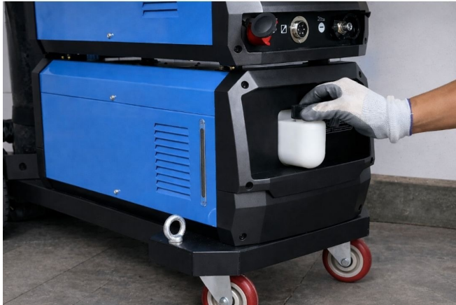
Fig. 5.3 Filling the coolant tank
