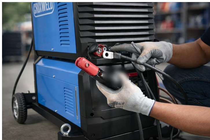
Fig. 5.2 Connecting a cable to the output terminal
