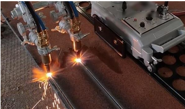
Dual torch oxy-fuel cutting
