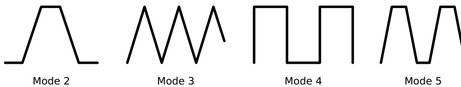
Swing modes 2 to 5 (mode 1 = no swing, straight travel)
