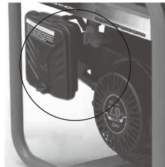
Fig. 4.2 Choke open (running)
