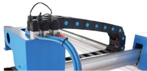
Fig. 7-2 Reinforced nylon drag chain and solenoid valves on the drive unit
