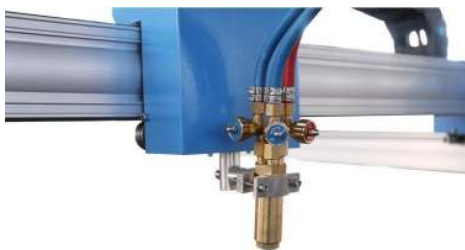
Fig. 7-1 Flame torch and gas manifold on the torch lifter
