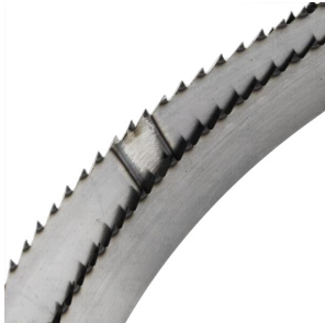
Finished weld joint
